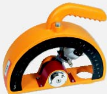
Type PT for 0,2 to 5 N/mm 2 , e.g. plaster, light-weight concrete.
